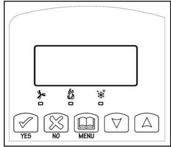
It is possible to bring up the user menu at any time by depressing the MENU key. The status display automatically resumes after exiting the user-configuring menu.
