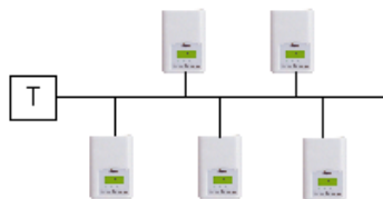
Figure 3.1 Singly Terminated Bus Topology
