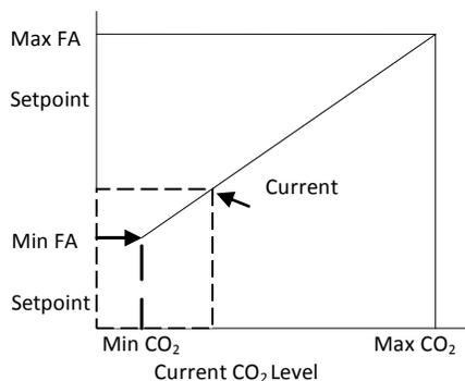
The highest value between free cooling demand output and interpolation output for the fresh air setpoint based on the CO<sub>2</sub> level will be the output to the fresh air damper
