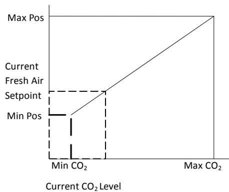
The highest value between free cooling demand output and interpolation output for the fresh air setpoint will be the output to the fresh air damper.
